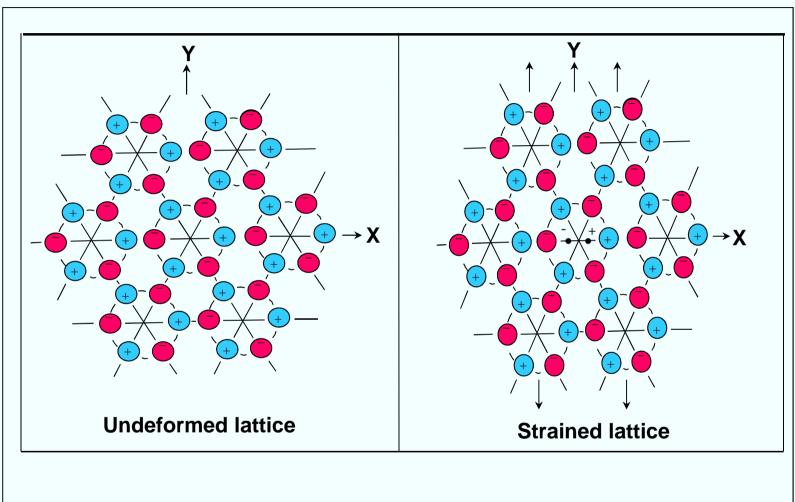
The piezoelectric effect provides a coupling between the mechanical properties of a piezoelectric crystal and an electrical circuit.
