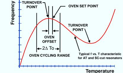
Oven Parameters vs. Stability for SC-cut Oscillator Assuming  $T_i - T_{LTP} = 10^{\circ}C$
