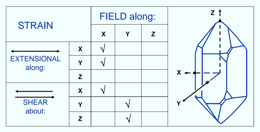
In quartz, the five strain components shown may be generated by an electric field. The modes shown on the next page may be excited by suitably placed and shaped electrodes. The shear strain about the Z-axis produced by the Y-component of the field is used in the rotated Y-cut family, including the AT, BT, and ST-cuts.
