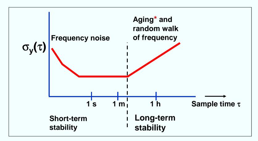
\*For  $\sigma_y(\tau)$  to be a proper measure of random frequency fluctuations, aging must be properly subtracted from the data at long  $\tau$ 's.
