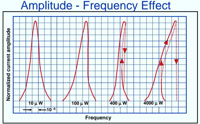
At high drive levels, resonance curves become asymmetric due to the nonlinearities of quartz.
